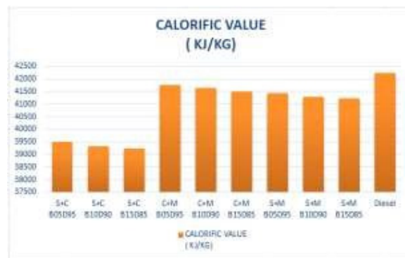
Figure 6 Calorific values of different Biodiesel blends.
