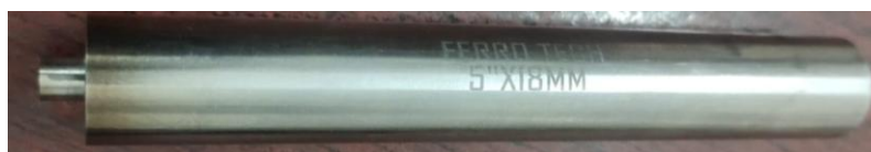
Figure 2.4: FSW Cylindrical Pin Profile Tool - HSS
