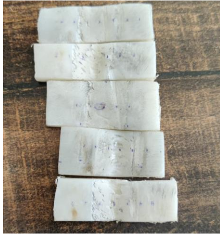
Figure 2.9: Rockwell-M Hardness Test Specimens
