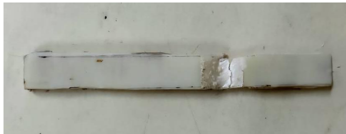
Figure 2.11: Izod Impact Fractured Specimen
