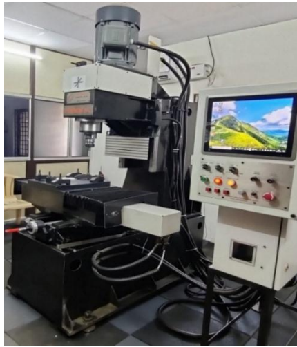
Figure 2.2: CNC-Controlled Friction Stir Welding (FSW) Machine (JNTU-H)
