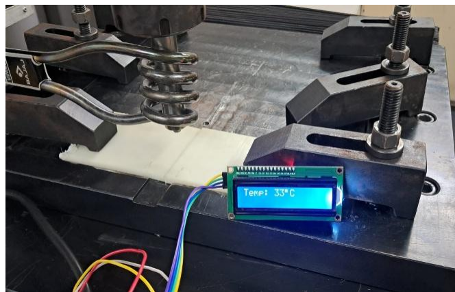
Figure 2.7: Induction System Setup on FSW Machine
