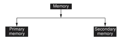
When the main memory holds instruction and data when a program is executing the auxiliary memory or secondary memory holds data and programs which are not intently in use and furnishes long term storage.
