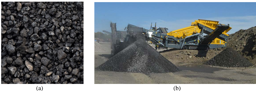
Fig.1 (a) Recycled Asphalt Pavement (b) Processing of RAP into Fine and Coarse Aggregate
