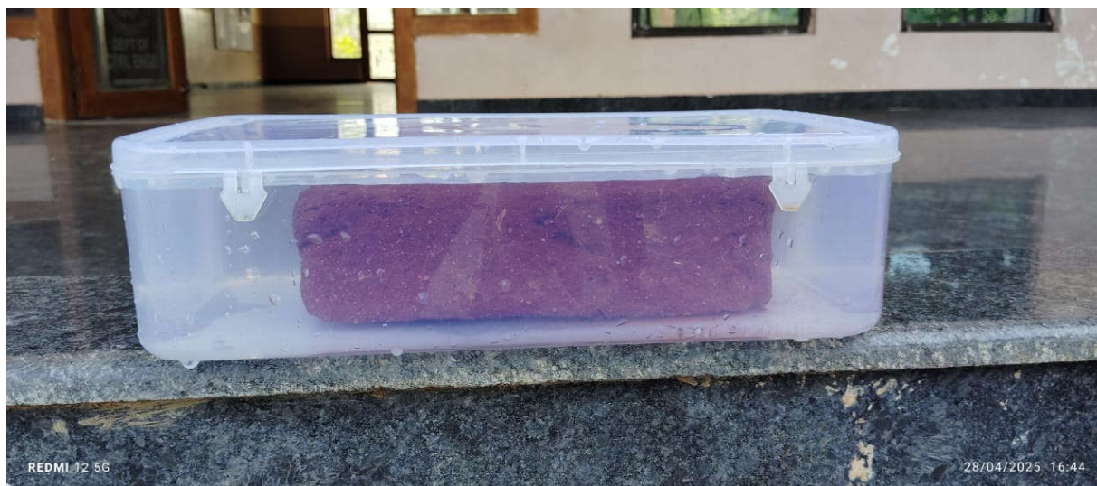
Fig. 2 Brick specimen's submergence in the leaching solution following the NEN standards
